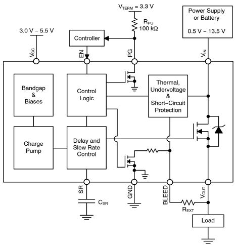
Figure 3. Typical Application Diagram - Load Switch
