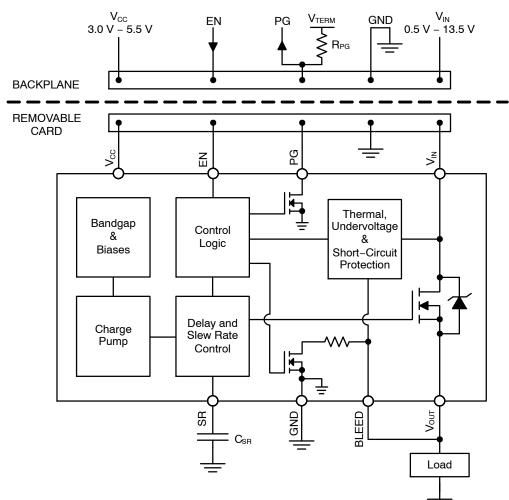
Figure 4. Typical Application Diagram - Hot Swap
