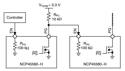
Figure 5. Simplified Application Diagram - Power Sequencing with PG Output
