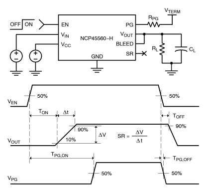
Figure 2. Switching Characteristics Test Circuit and Timing Diagrams
