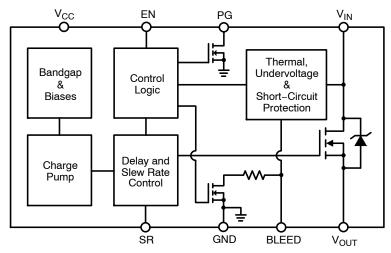
Figure 1. Block Diagram
